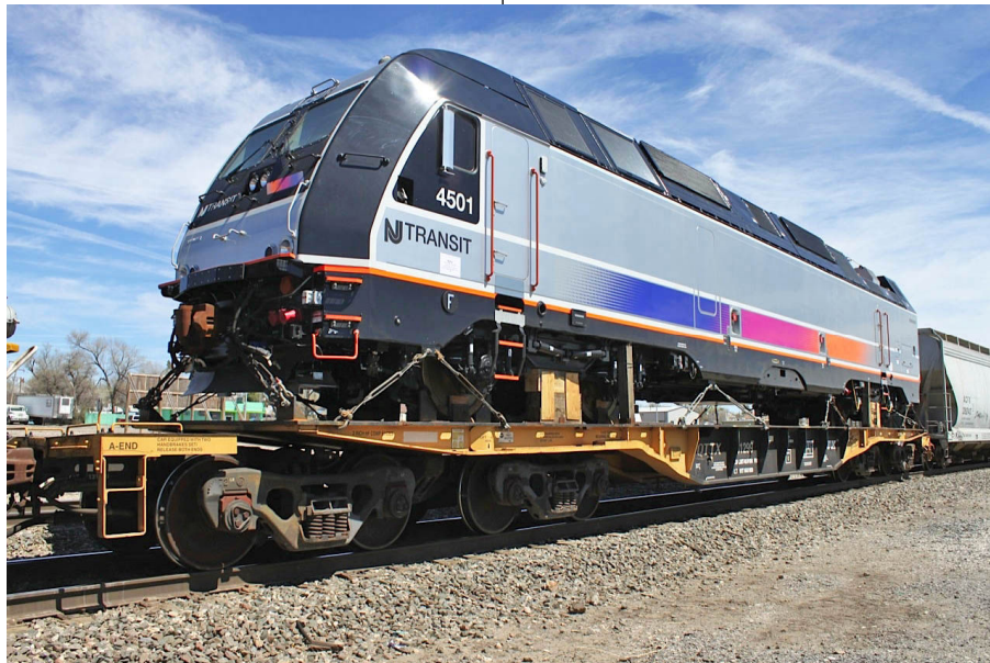
New Jersey Transit 4501 on the H-KCKDEN1-05 at Dodge City April 5. The ALP-45DP is a dual-mode locomotive built at Bombardier and is en route the Transportation Technology Center at Pueblo, Colorado. NJT has 26 of these units on order. Photo by David Webb.
